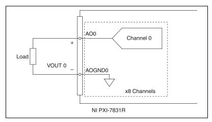
Figure 2-9. Analog Output Connections
